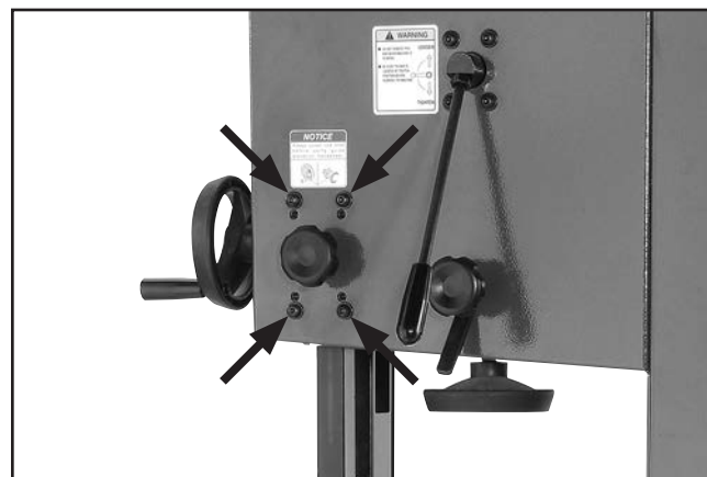
Figure 102. Guide post adjustment screws.
