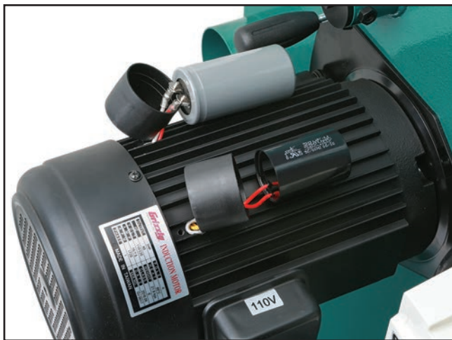
Figure 119. Start and run capacitors.
