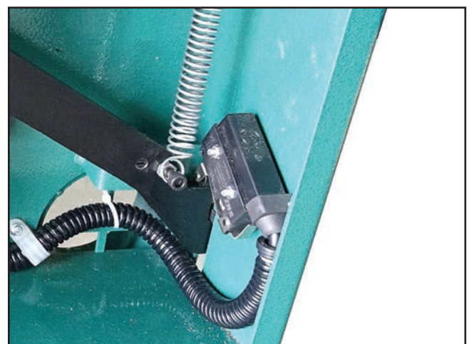
Figure 123. Foot brake limit switch.
