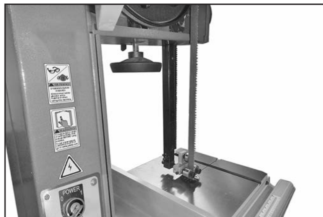
Figure 104. Guide post guard removed.
