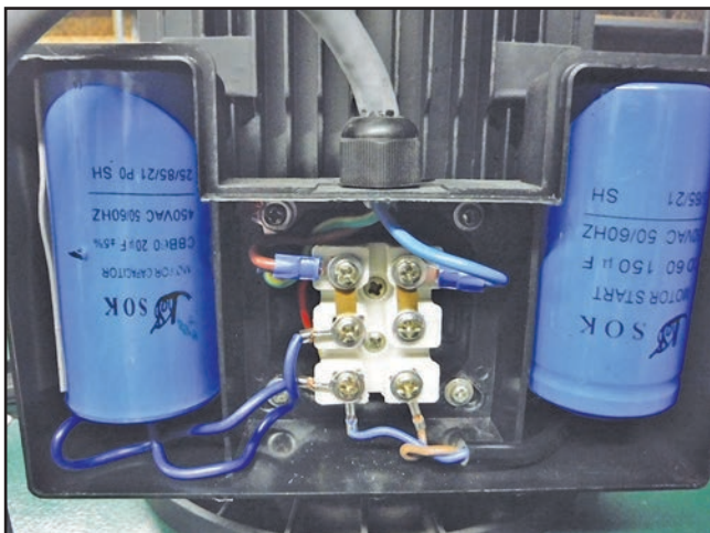
Figure 39. Motor and capacitor wiring.
