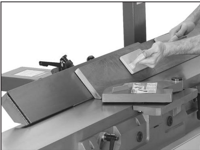
Figure 39. Example of fence setup for a bevel cut of 45°.
