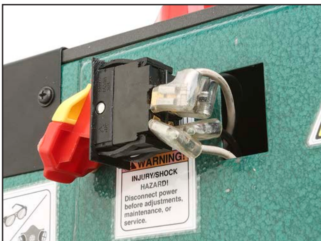
Figure 62. G0821 switch wiring.
