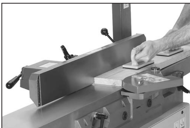
Figure 34. Example of surface planing operations.
