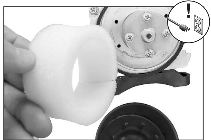
Figure 70. Typical air pump foam filter.
