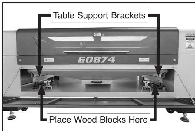
Figure 85. Z-axis table support brackets location (G0874 shown).
