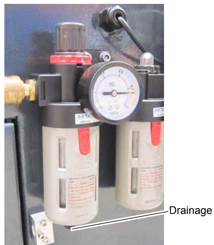
Img.11-2: Compressed air service unit
