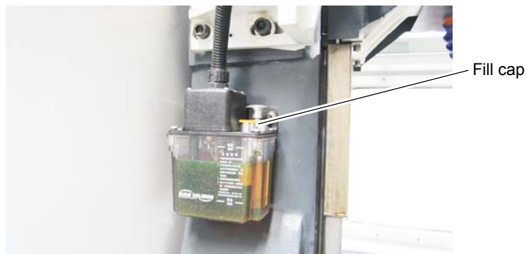
Img.3-4: Old type of central lubricating system
