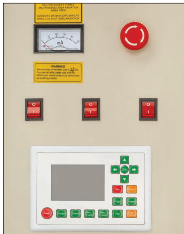
Figure 142. Control panel and power controls (G0911/G0912 shown).
