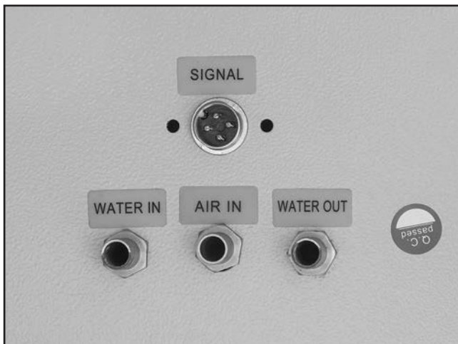
Figure 18. Water and air fittings for auxiliary systems connections (G0911/G0912 shown).
