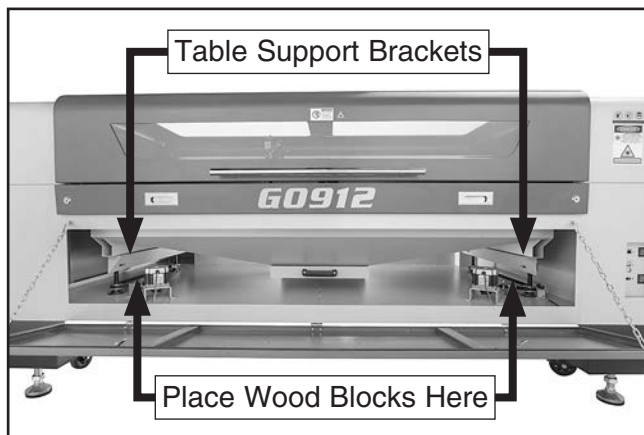
Figure 87. Z-axis table support brackets location.
