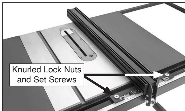
Figure 119. Location of lock nuts and set screws for adjusting fence squareness and height.
