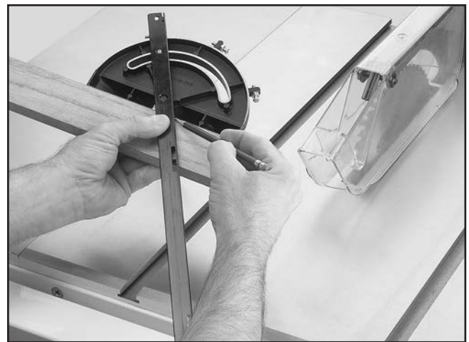
Figure 59. Example of marking miter line.
