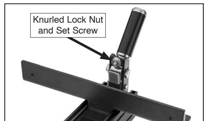
Figure 124. Set screw for adjusting fence handle clamping pressure.
