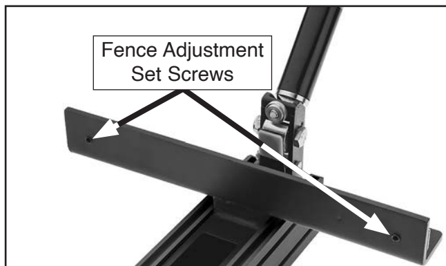
Figure 125. Location of set screws to adjust fence parallelism (shown upside down).
