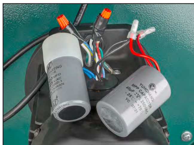
Figure 46. Motor junction box wiring (120V).
