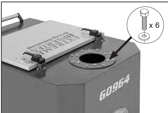
Figure 15. Location of precision arm fasteners.
