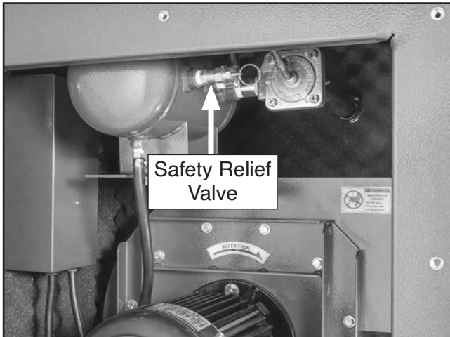
Figure 28. Location of safety relief valve.
