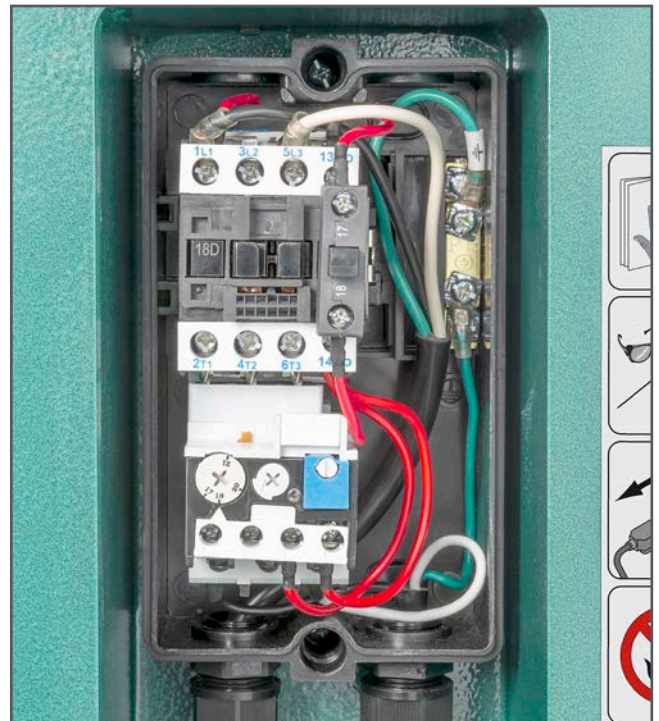
Figure 48. Magnetic switch wiring (120V).
