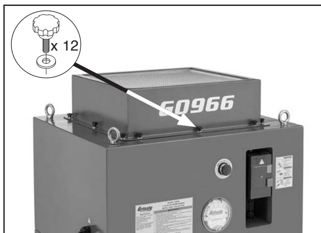
Figure 7. Location of HEPA filter cage knob bolts.
