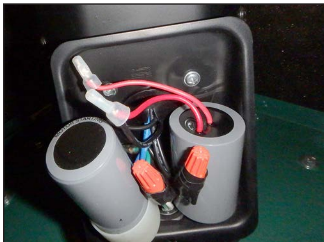
Figure 47. Motor junction box wiring (120V).
