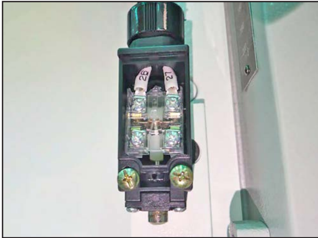
Figure 134. Upper elevation limit switch (LS1).
