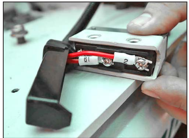
Figure 138. Dust hood safety switch (LS5).
