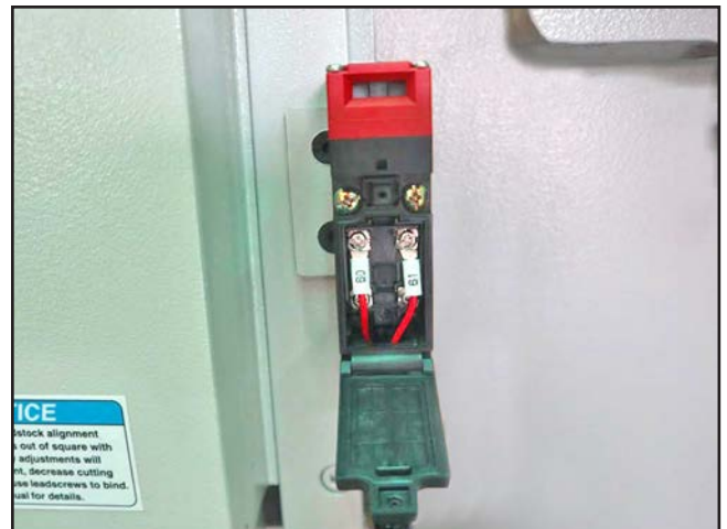
Figure 139. Belt guard safety switch (LS6).
