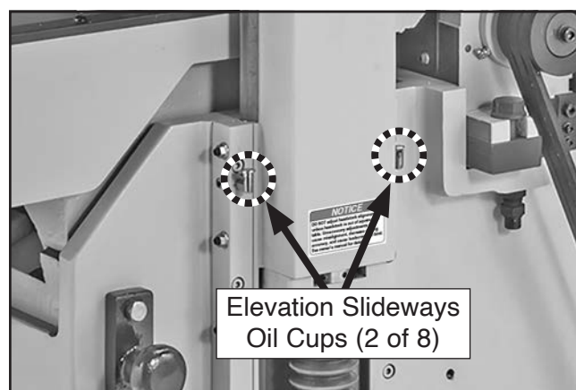
Figure 72. Location of elevation slideway oil cups (2 of 8).
