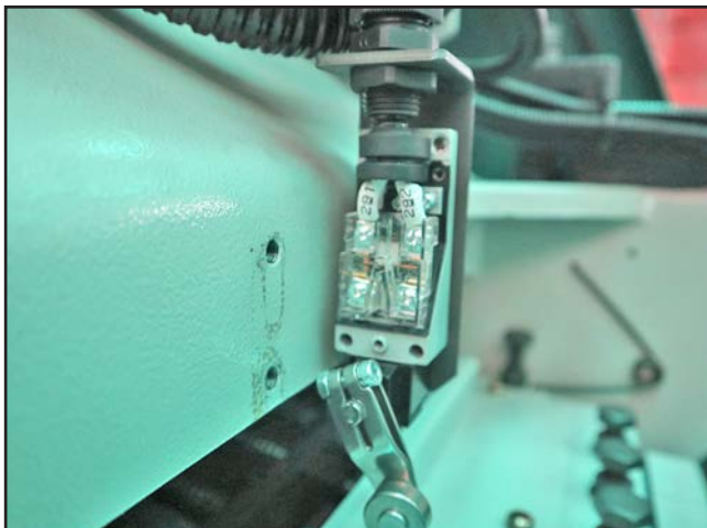
Figure 136. Chip breaker safety switch (LS3).
