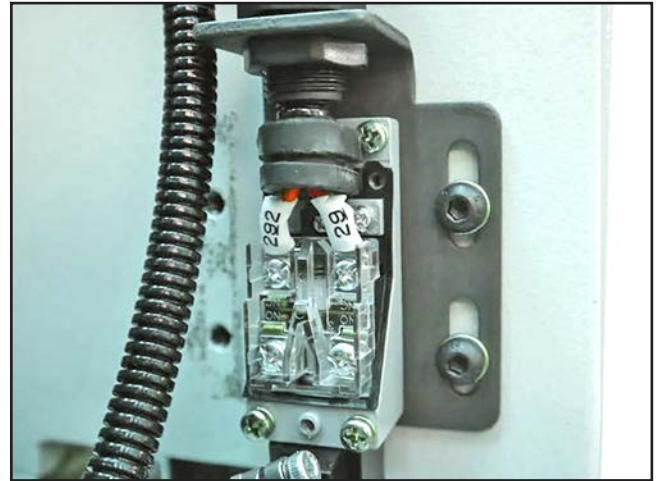
Figure 137. Pressure bar safety switch (LS4).
