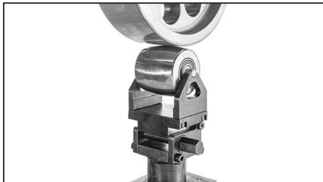
Figure 21. Lower wheel in operating position (workpiece removed for clarity).
