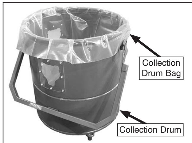
Figure 29. Collection bag placed in collection drum.
