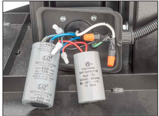
Figure 88. G0976 motor wiring.
