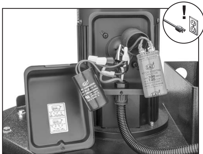
Figure 7. G0975 motor junction box.
