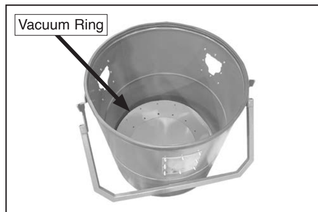
Figure 28. Vacuum ring placed inside collection drum.
