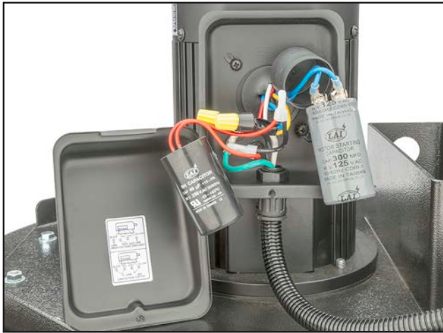
Figure 86. G0975 motor wiring.
