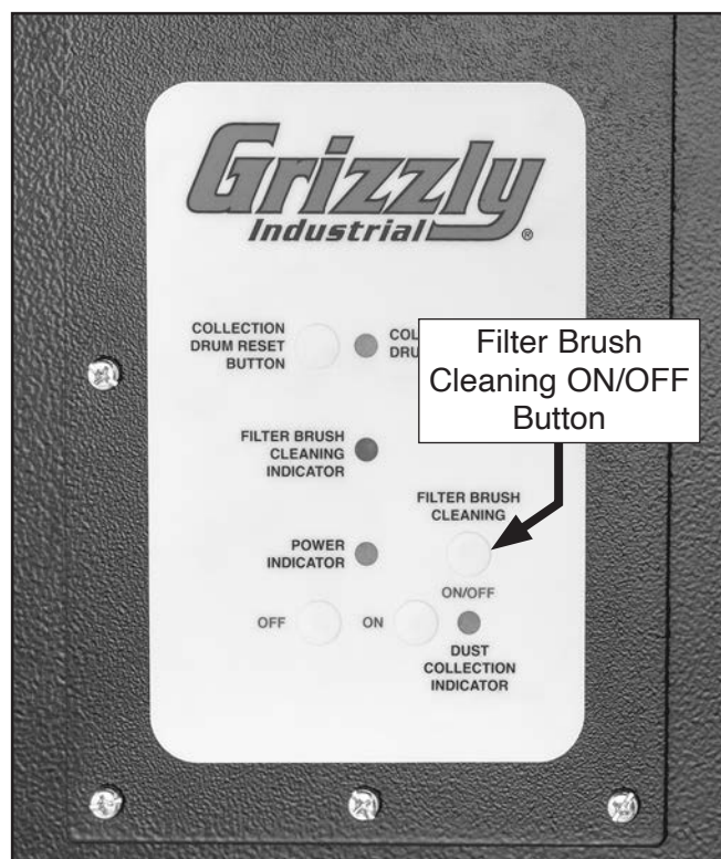
Figure 76. Location of filter brush cleaning ON/OFF button.
