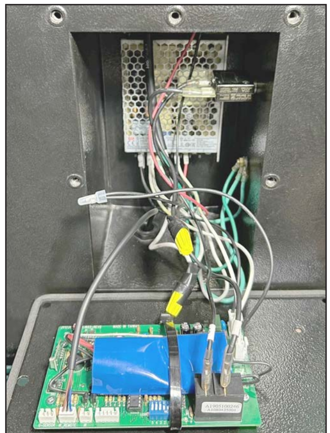
Figure 89. G0976 control panel wiring.
