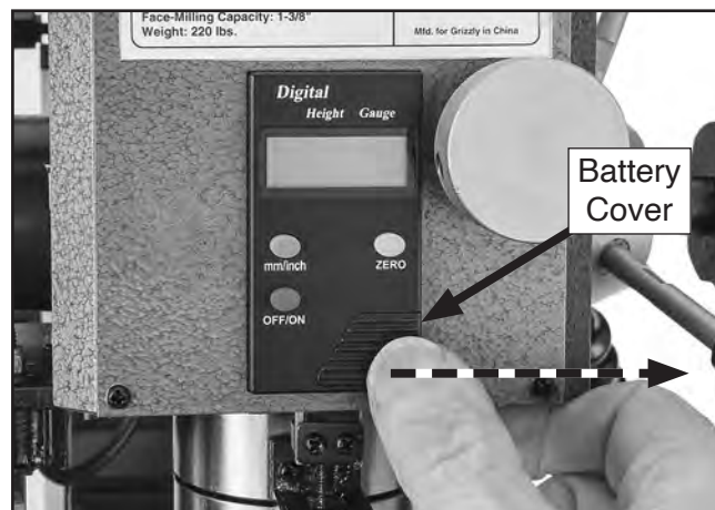
Figure 62. Example of removing spindle depth DRO battery cover.
