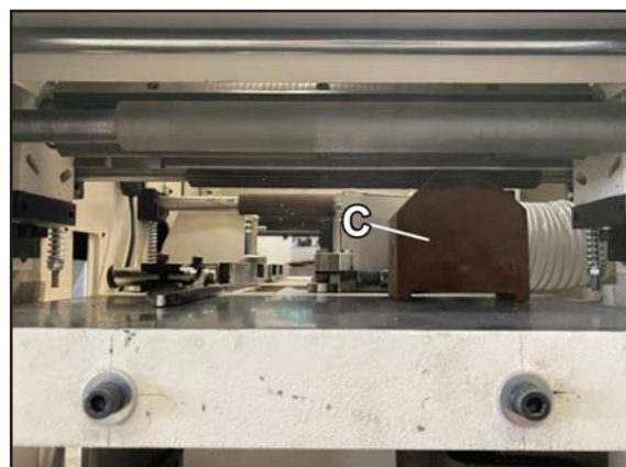
Figure 64. Gauge block placed below cutterhead.
