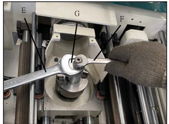
Figure 39. Removing cutterhead nut.
