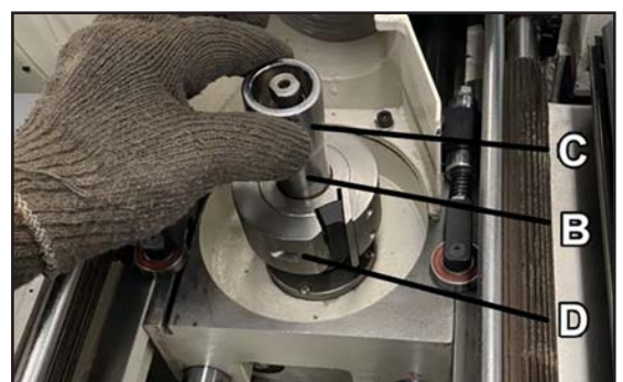
Figure 41. Placing spacers on top of cutterhead.
