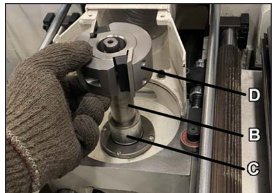
Figure 40. Placing cutterhead on top of spacers.
