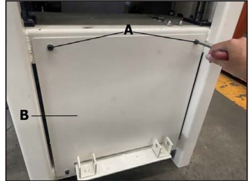
Figure 57. Location of rear cover and screws.
