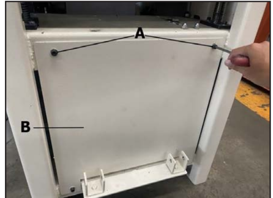
Figure 60. Location of rear cover screws.
