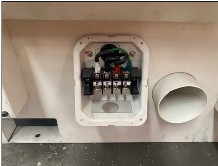
Figure 16. Location of ground and power terminals.
