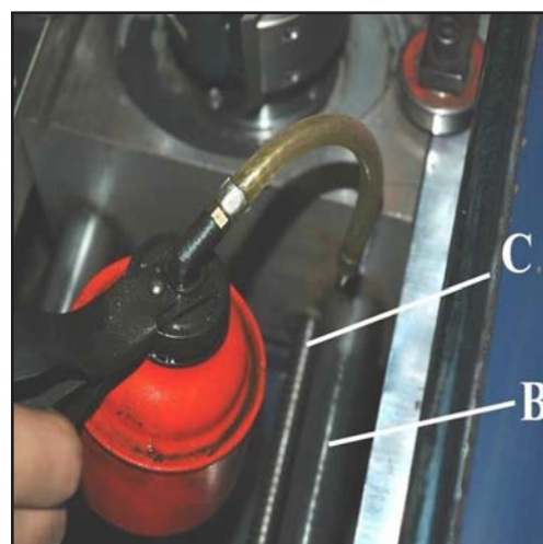
Figure 56. Lubricating table slide ways.
