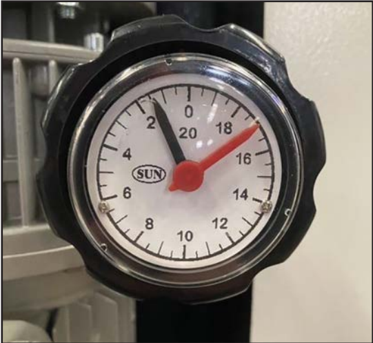
Figure 52. Feed speed adjustment knob reference scale.
