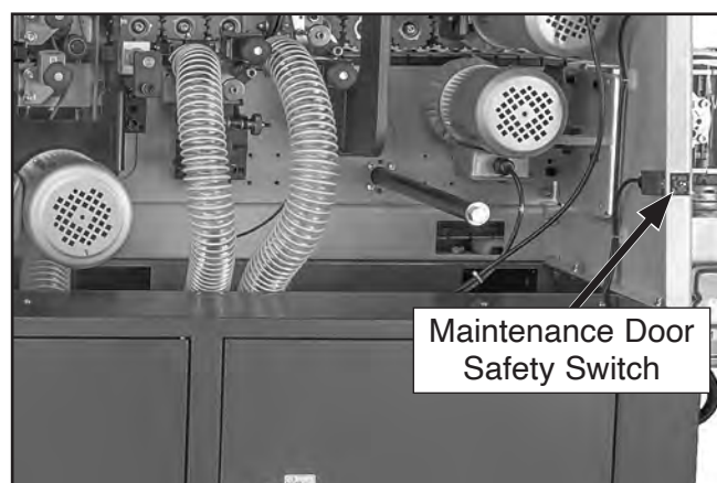
Figure 135. Location of maintenance door safety switch.
