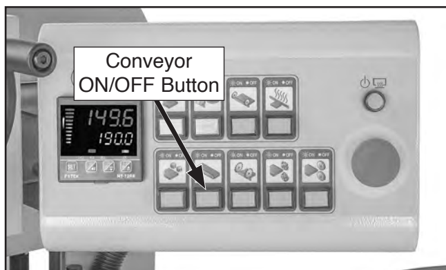
Figure 39. Location of conveyor ON/OFF button.
