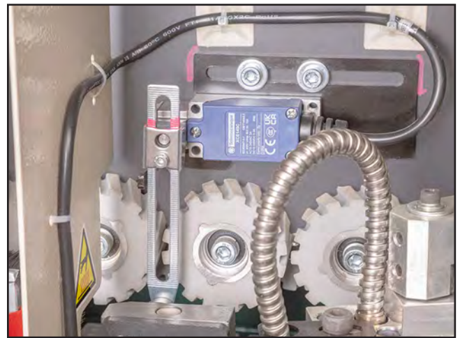
Figure 161. Edgebanding advancement/ guillotine limit switch.
