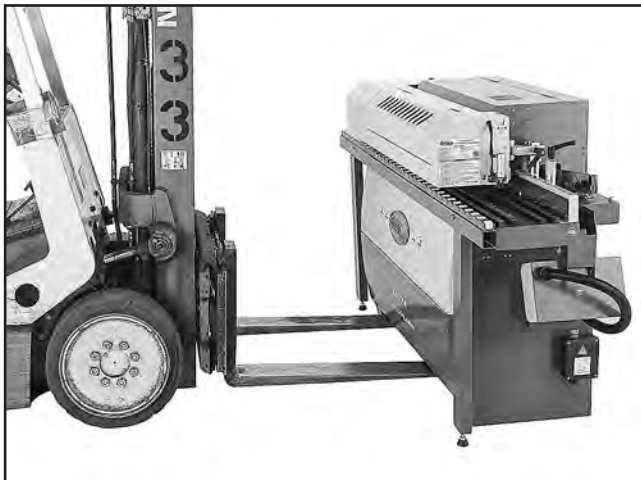
Figure 15. Example of inserting forks for lifting edgebander.
