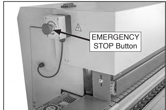
Figure 43. Location of outfeed EMERGENCY STOP button.
