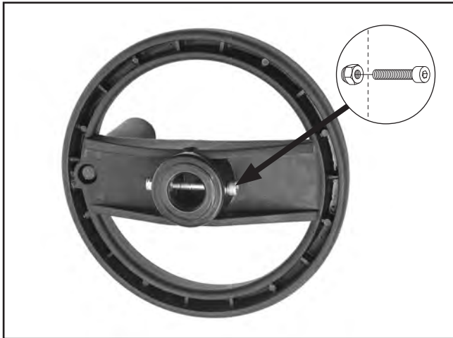
Figure 17. Location of pre-installed panel feeder height handwheel mounting hardware.
