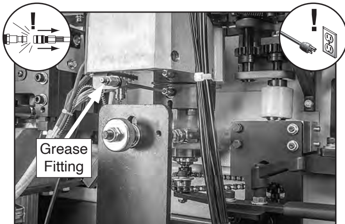
Figure 75. Location of glue spindle grease fitting (shield removed for clarity).
