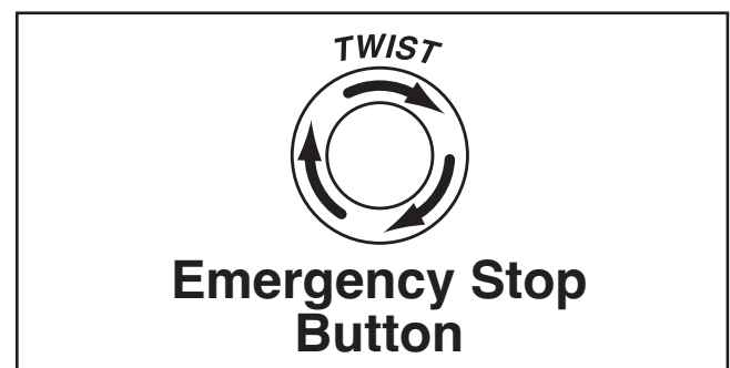
Figure 37. Resetting Emergency Stop button.
