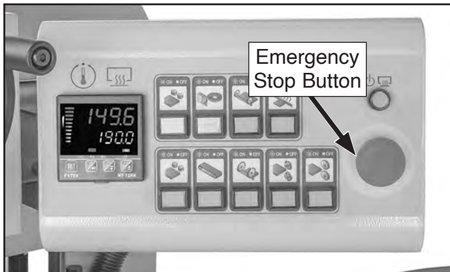
Figure 42. Location of control panel Emergency Stop button.
