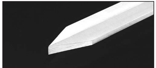
Figure 39. Parting tool example.
