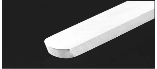
Figure 38. Round nose scraper example.
