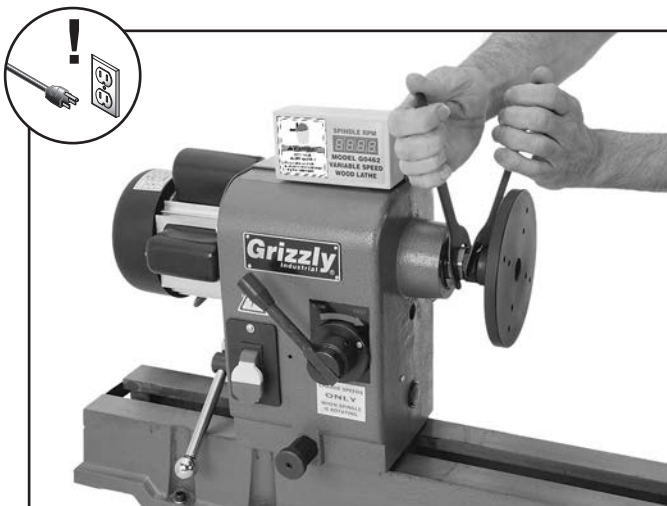
Figure 23. Example of loosening faceplate.
