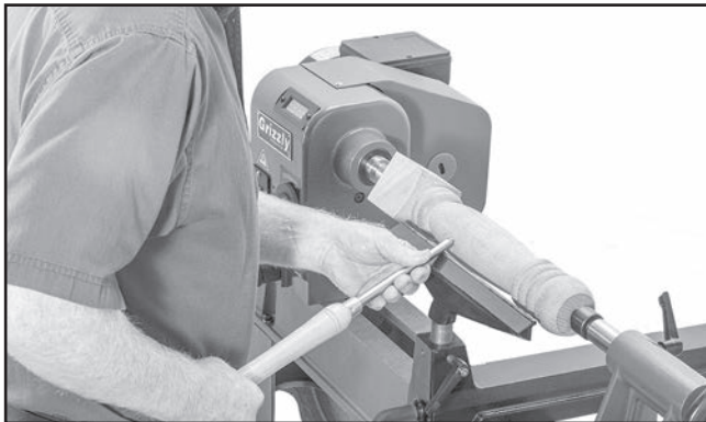
Figure 26. Typical spindle turning operation.
