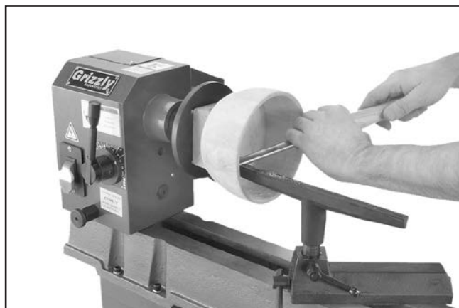
Figure 30. Typical faceplate turning operation.
