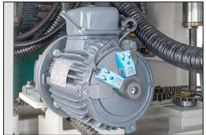
Figure 106. Table elevation motor sensor wiring.
