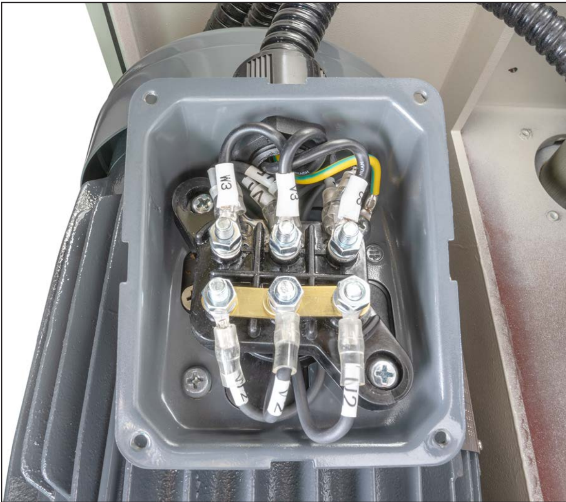
Figure 114. Feed motor wired for 220V operation.
