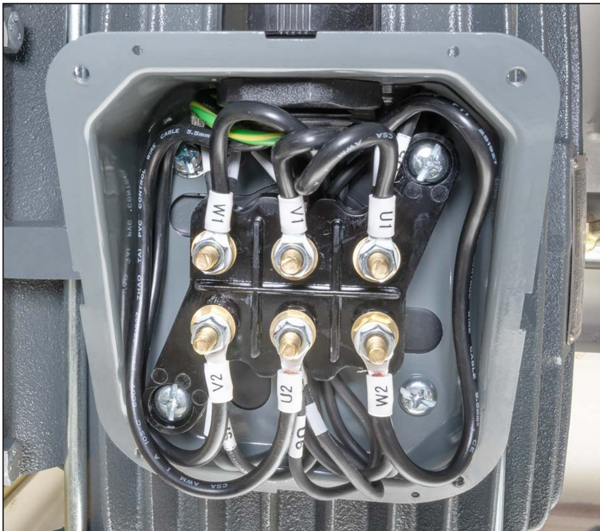
Figure 115. Cutterhead motor wired for 220V operation.
