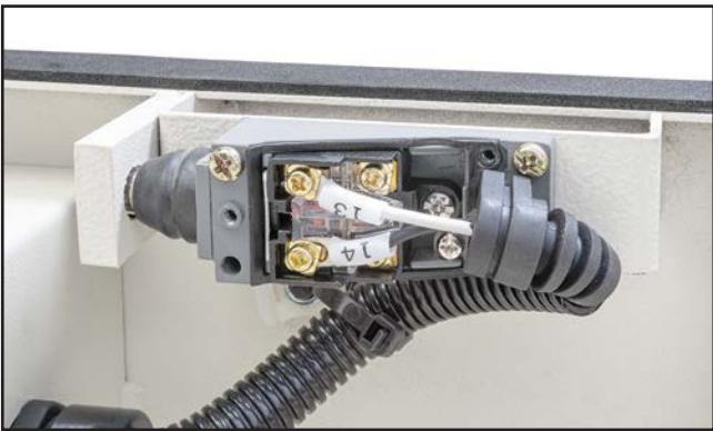
Figure 111. Top cover limit switch wiring.
