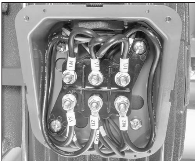
Figure 22. Cutterhead motor wiring (220V).
