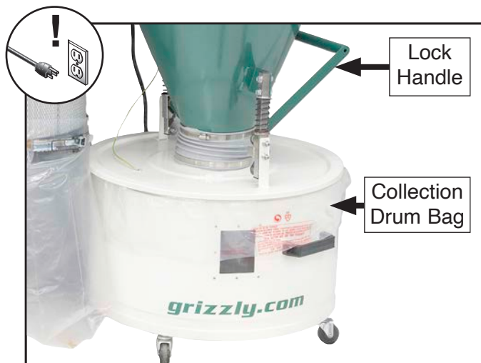
Figure 57. Collection drum bag components.
