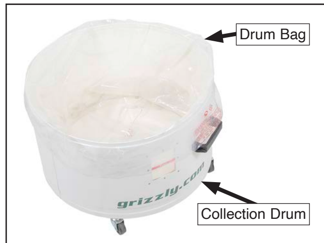
Figure 20. Collection drum bag installed.
