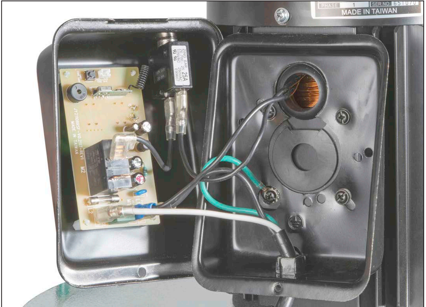
Figure 71. Motor junction box wiring.
