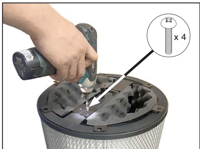
Figure 64. Removing sound dampening wedge fasteners.
