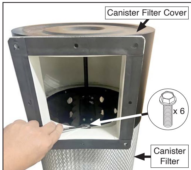
Figure 67. Tightening flange bolts on canister filter cover.
