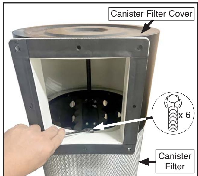
Figure 62. Loosening flange bolts on canister filter cover.
