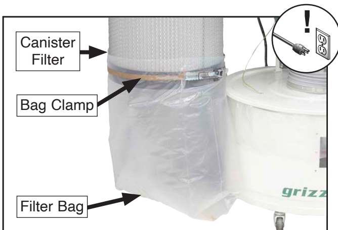
Figure 60. Location of filter bag and bag clamp.
