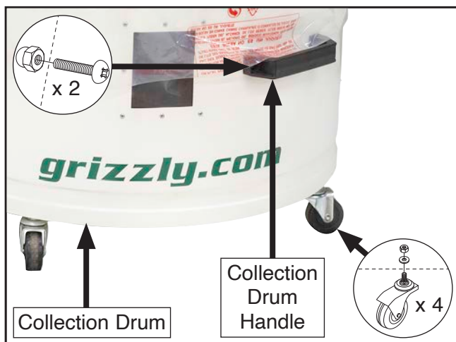
Figure 19. Casters and collection drum handle attached to collection drum.
