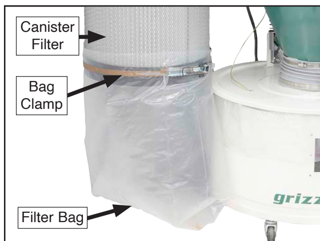
Figure 70. Filter bag attached to canister filter.
