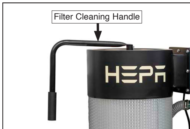
Figure 69. Location of filter cleaning handle.
