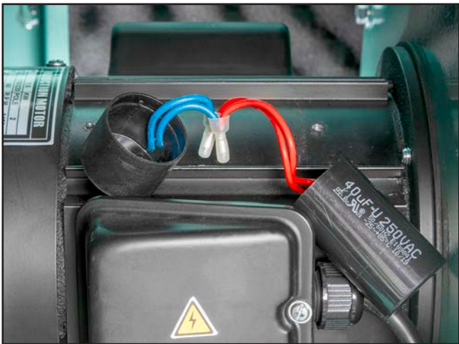
Figure 67. Run capacitor wiring.
