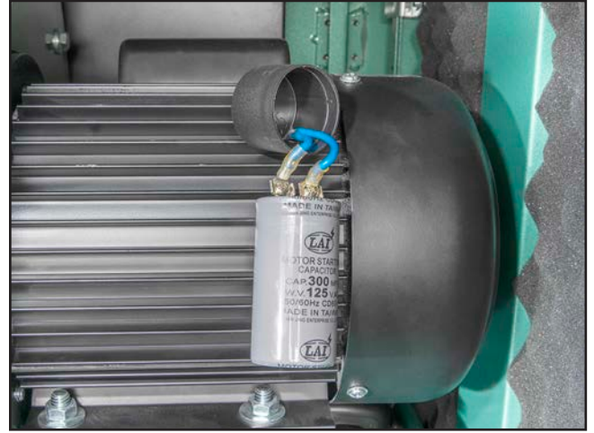
Figure 68. Start capacitor wiring.
