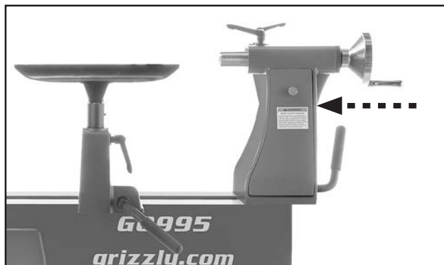
Figure 20. Installing tailstock on bed.
