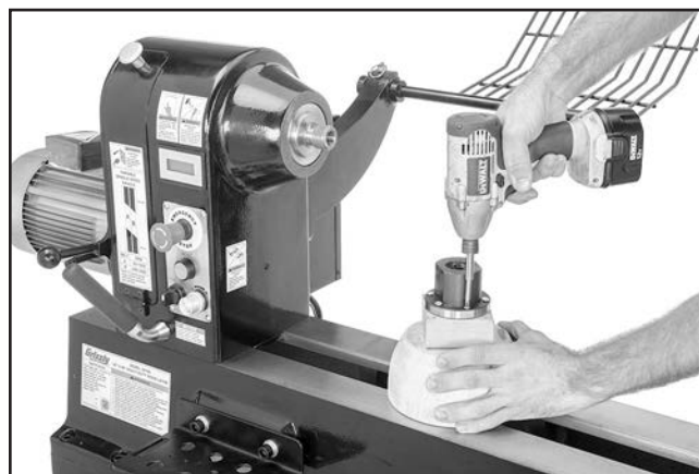
Figure 84. Typical attachment of faceplate to workpiece.
