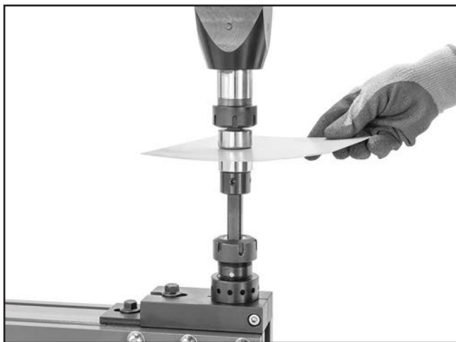
Figure 37. Example of anvil die height adjusted to workpiece thickness.
