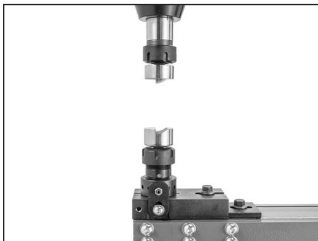
Figure 32. Anvil die oriented to align with hammer die (louver dies shown).
