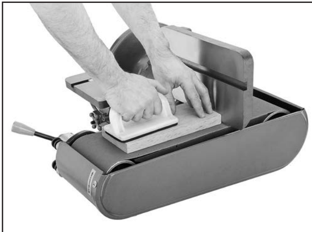
Figure 41. Example of face sanding with platen in horizontal position.
