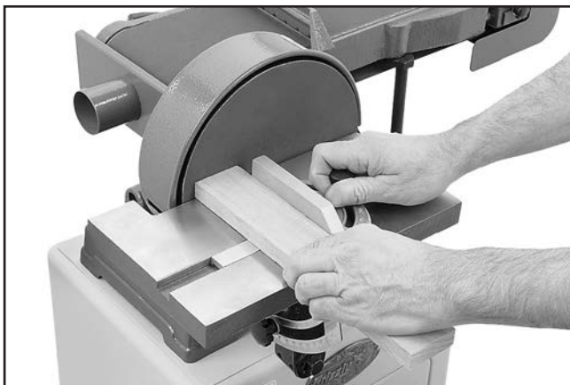
Figure 34. Example of 90° disc sanding.
