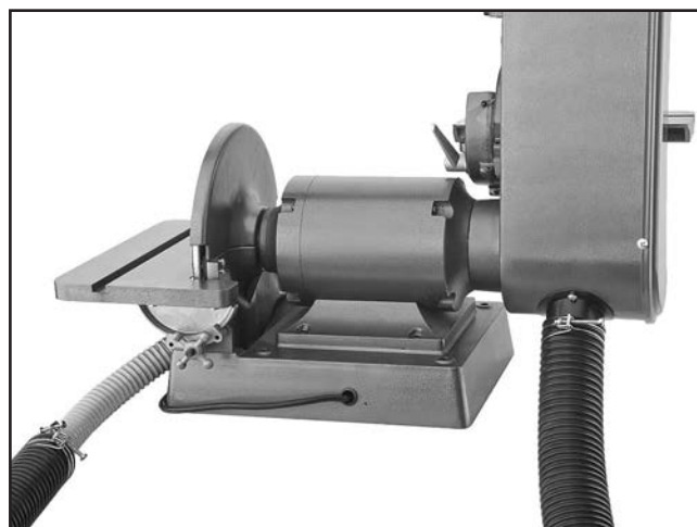
Figure 23. Example of hoses attached to ports.
