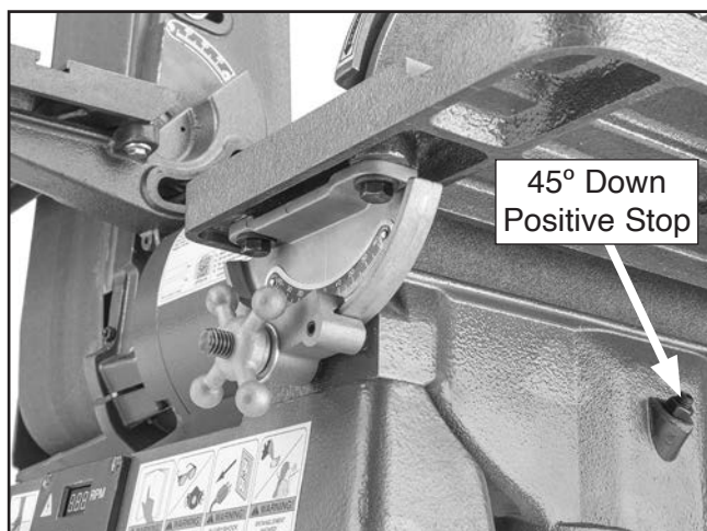
Figure 30. Sanding disc table 45° down positive stop.
