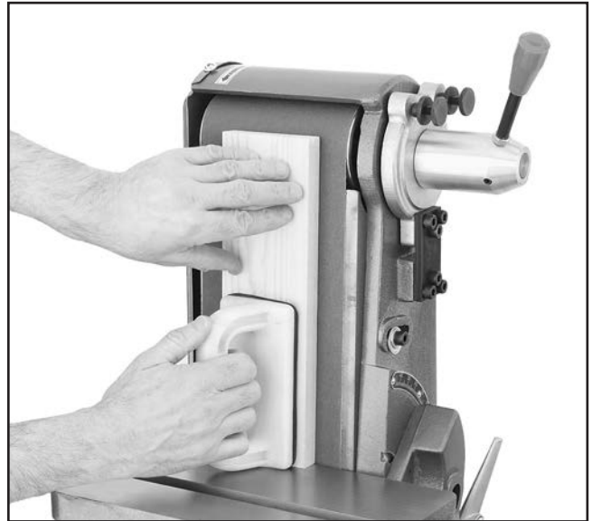
Figure 42. Example of face sanding with platen in vertical position.
