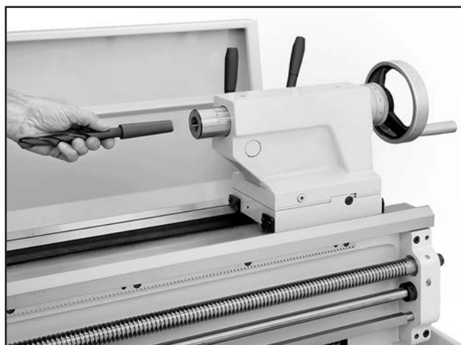
Figure 49. Example of inserting tapered tool into tailstock.
