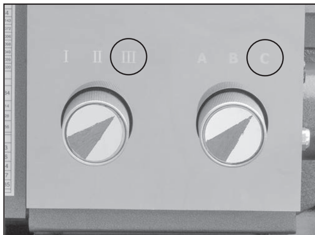
Figure 97. Gearbox dials positioned for 16 TPI.
