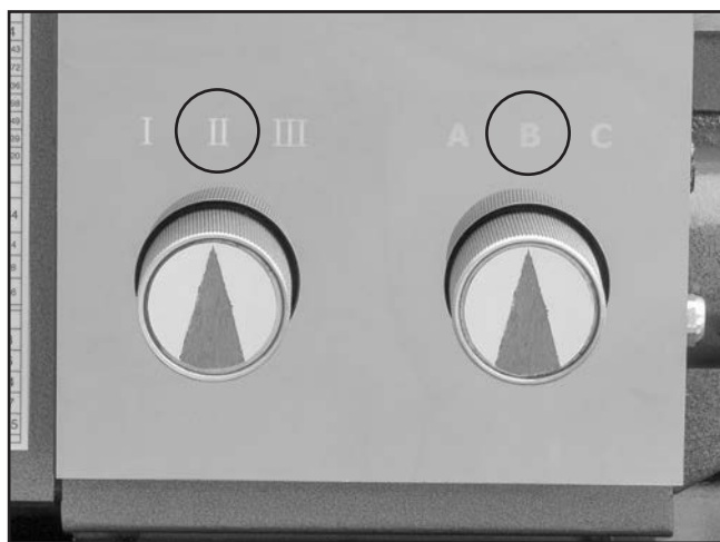
Figure 81. Gearbox dials positioned for 0.0049 in./rev. cross slide feed rate.
