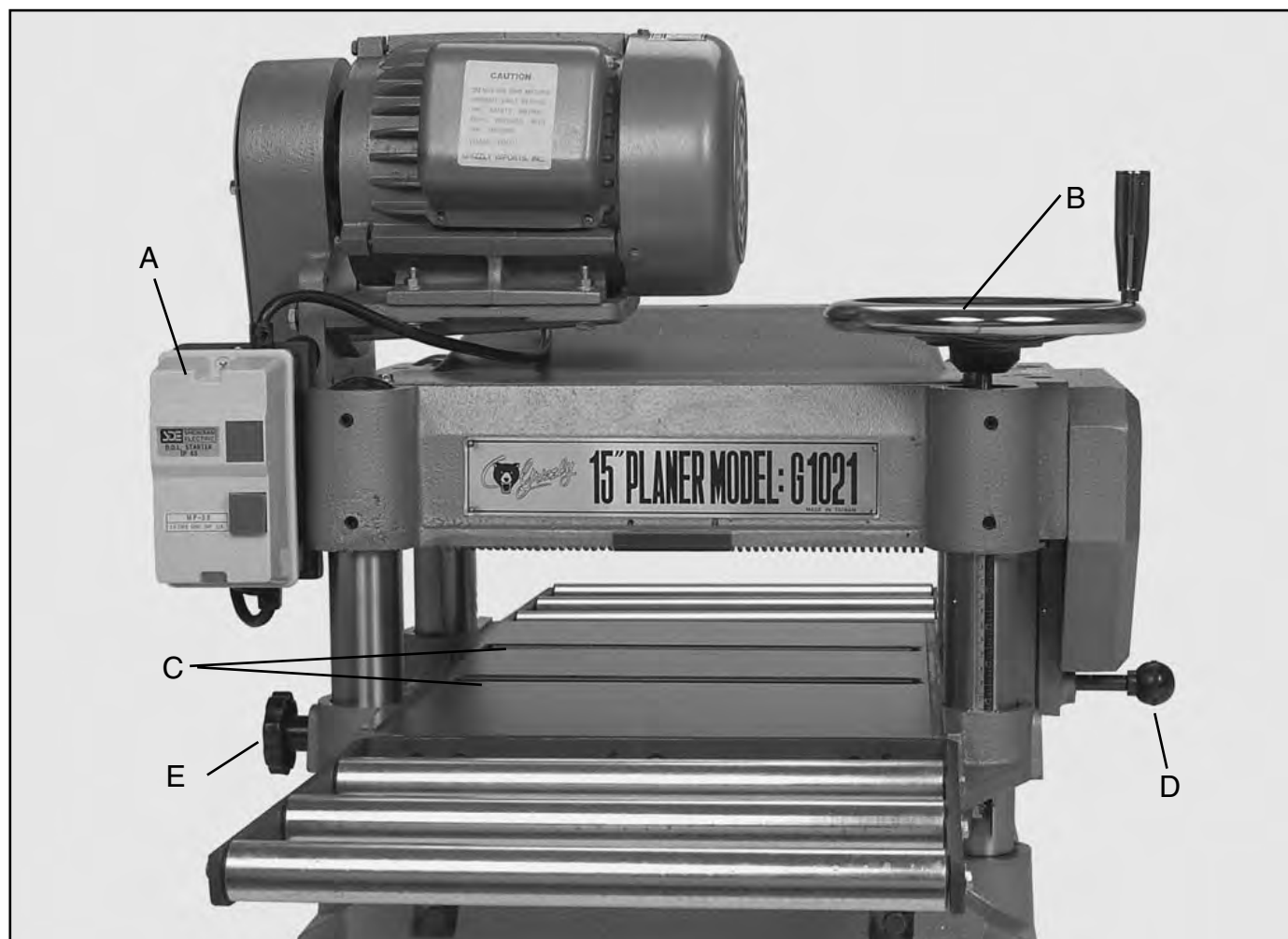
Figure 10. Overview of planer adjustment controls.
