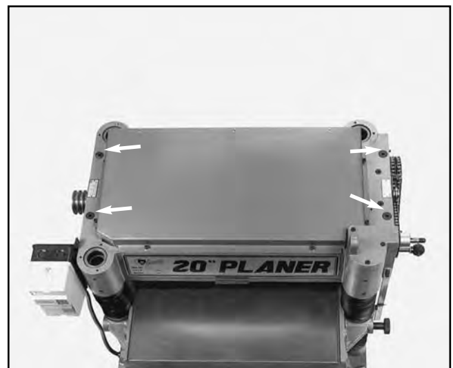
Figure 41. Feed roller lubrication points.
