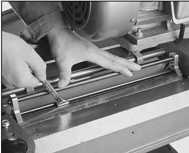
Figure 16. Tightening knives in cutterhead.
