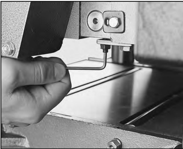
Figure 20. Feed roller height adjustment.
