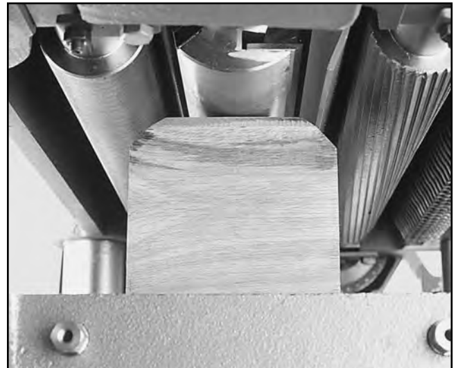
Figure 12. Guide block indicates parallelism.
