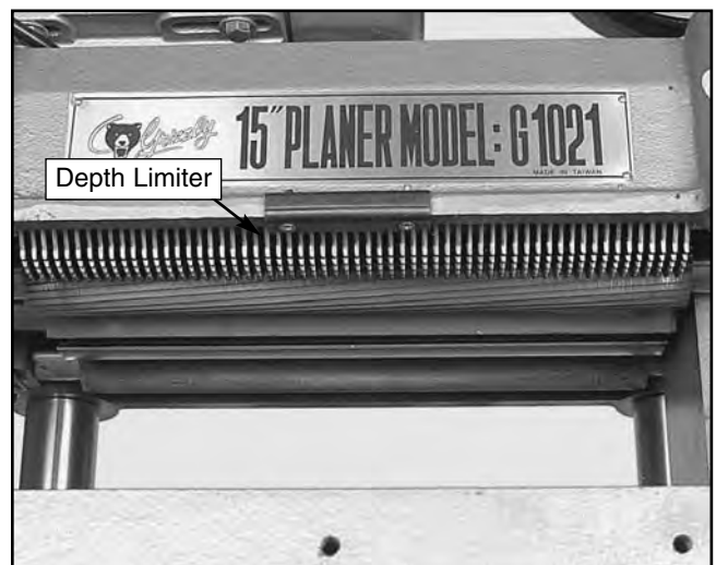
Figure 36. Location of depth limiter.
