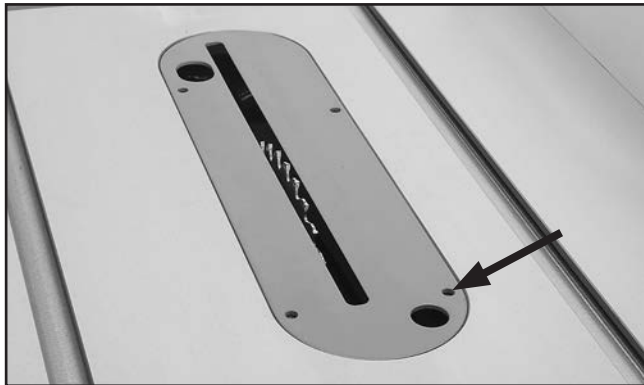
Figure 128. Location of table/dado insert holes with adjustment screws.
