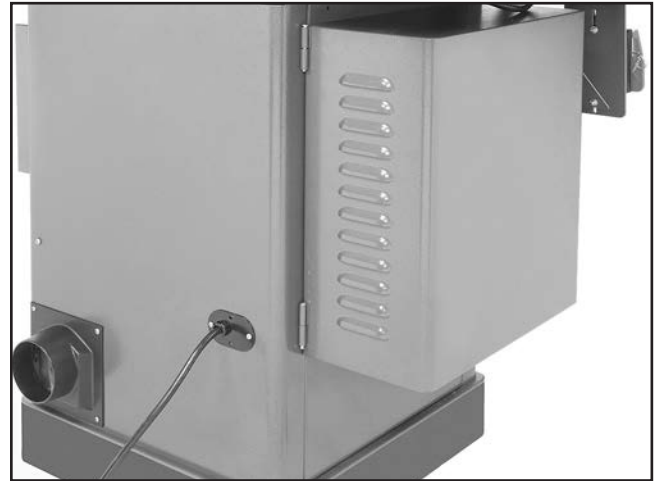
Figure 23. Motor cover installed.
