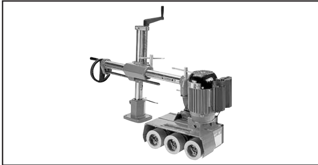
Figure 92. G4179 Power Feeder.
