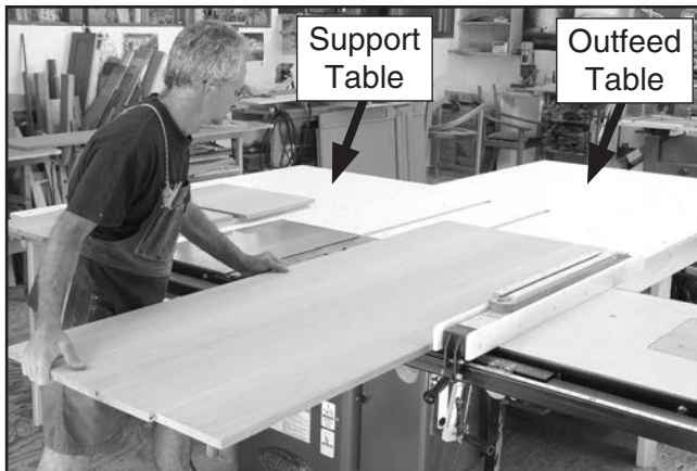
Figure 87. Example of outfeed & support tables.
