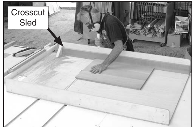
Figure 88. Example of crosscut sled.
