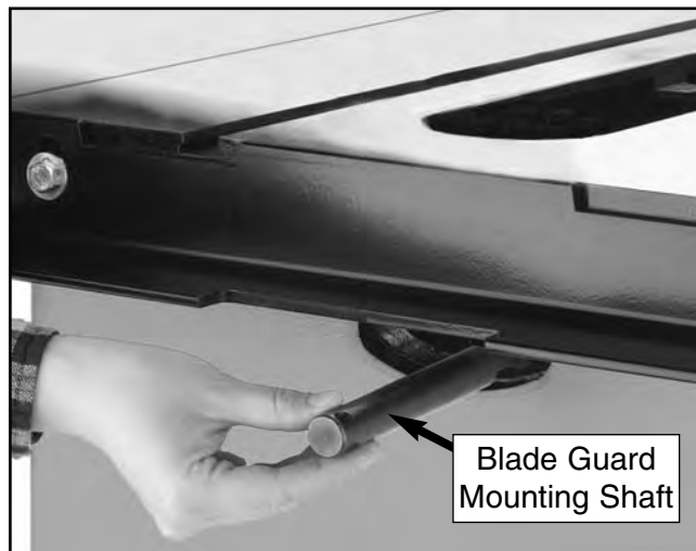
Figure 13. Attaching the \frac{5}{8} "-18 blade guard mounting shaft.
