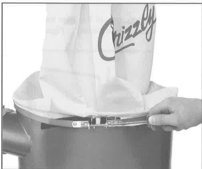
Figure 10. Tightening steel band.
