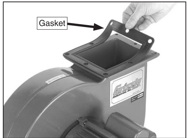
Figure 13. Positioning impeller outlet gasket.
