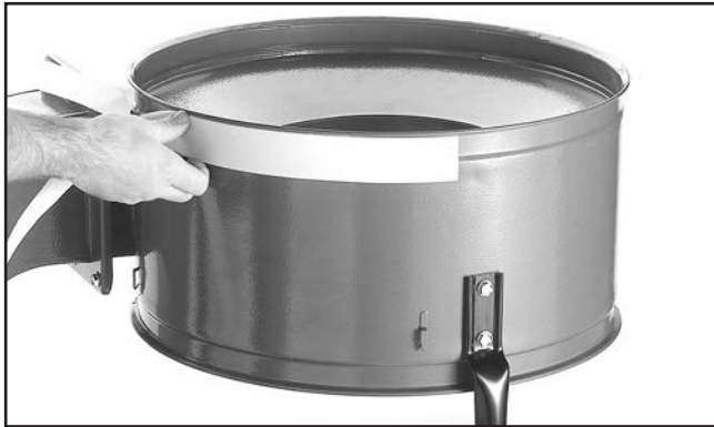
Figure 19. Installing wide foam strip.
