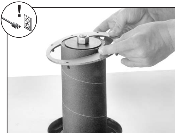
Figure 24. Installing table insert.
