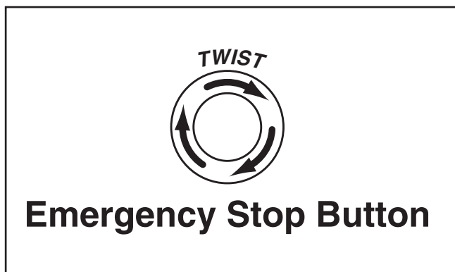
Figure 6. Resetting Emergency Stop button.
