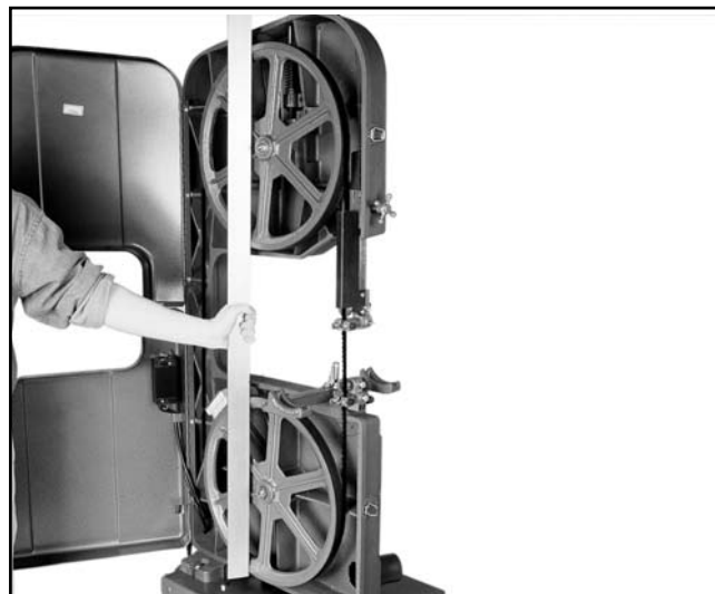
Figure 29. Holding a straightedge across both wheels.
