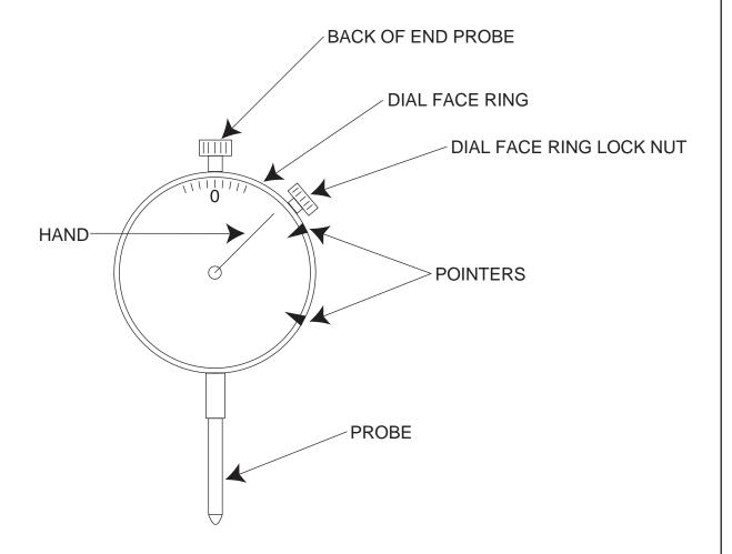
WHEN THE PROBE CONTACTS WORK PIECE OR OBJECT TO BE INDICATED, IT MOVES UP AND ROTATES THE HAND. TO ZERO HAND, LOOSEN DIAL FACE RING LOCKNUT. THEN TURN DIAL FACE RING UNTIL ZERO LINES UP WITH HAND. THEN YOU MAY TIGHTEN DIAL FACE RING LOCKNUT. THE POINTERS CAN BE MOVED INDEPENDENTLY TO SHOW ACCEPTABLE LIMITS OF TOLERANCE.
