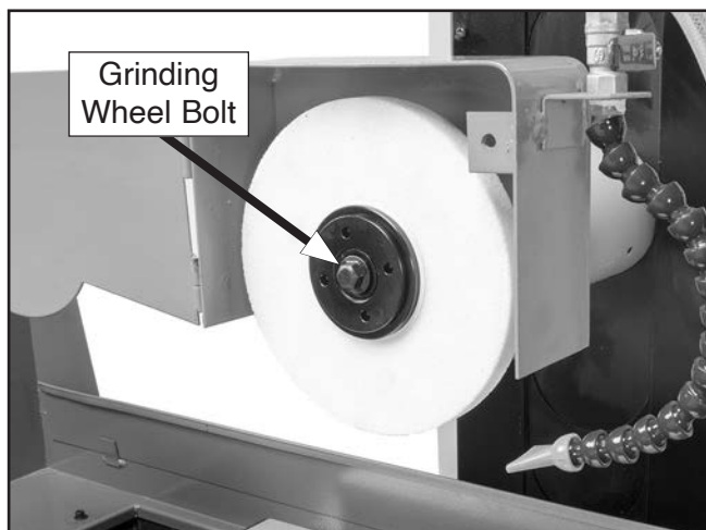
Figure 45. Wheel and grinding wheel bolt installed.
