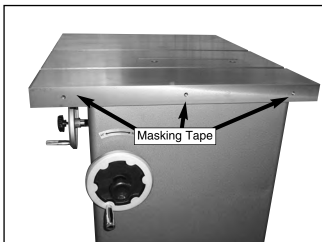
Figure 7. Using tape to shim for wing alignment.
