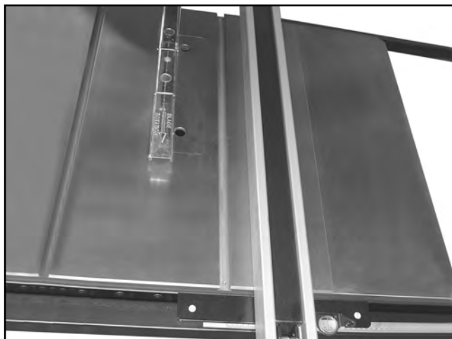
Figure 28. Fence aligned parallel to miter slot.
