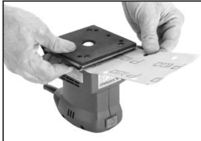
Figure 3. Attaching sandpaper on one side.
