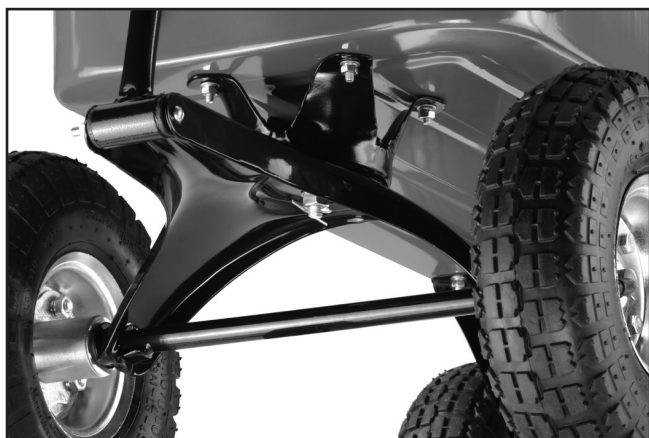
Figure 3. Steering bracket and front axle assembly mounted to the bed.
