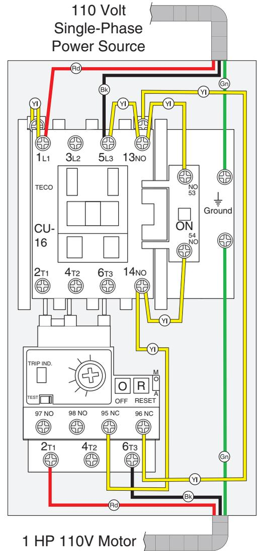
**IMPORTANT:** This magnetic switch toggles a motor ON and OFF, and helps provide thermal overload protection for the motor if the operating temperature gradually increases due to heavy work loads. The thermal overload relay inside is not designed to cut power in the event of a sudden motor overload or stall. To help protect a motor from this type of overload, the power supply circuit must be properly sized for the full-load current rating of the motor.
