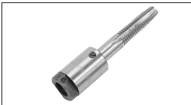
Figure 9. Tap installed into adapter.
