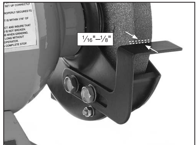
Figure 10. Work rest gap.
