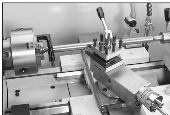
Figure 52. Generic picture of a workpiece mounted between dead centers.
