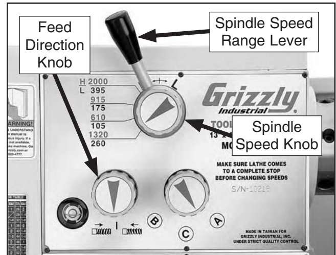
Figure 21. Headstock controls.
