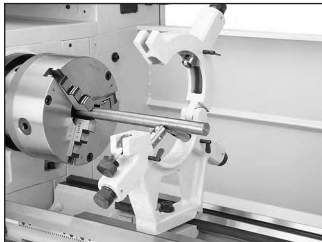
Figure 64. Generic picture of workpiece positioned in a typical steady rest.
