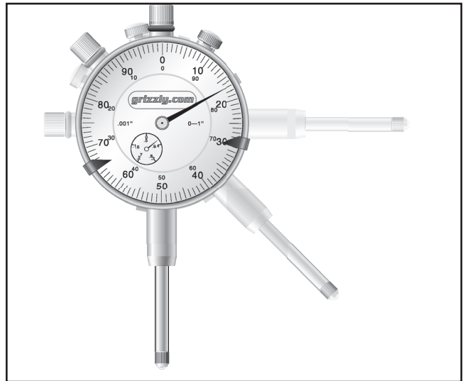
Figure 6. The indicator can be oriented in any direction by loosening the mounting stud , loosening the boom and raising the boom along the column .
