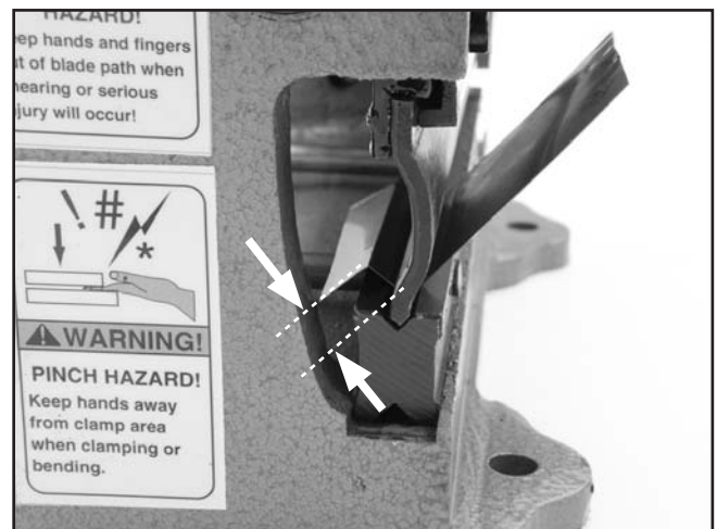
Figure 17. Minimum reverse bend.
