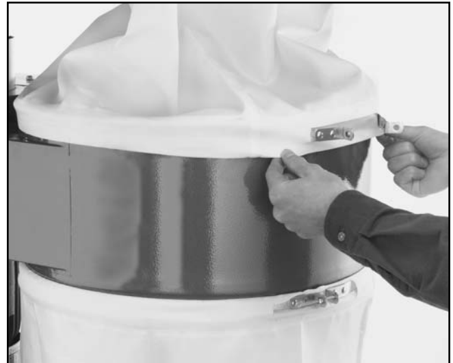
Figure 11. Attaching dust bags.
