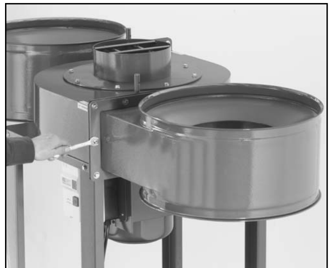
Figure 8. Attaching the collectors.
