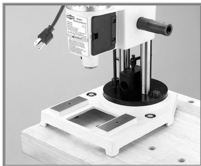
Figure 8. Machine positioned near edge of bench.
