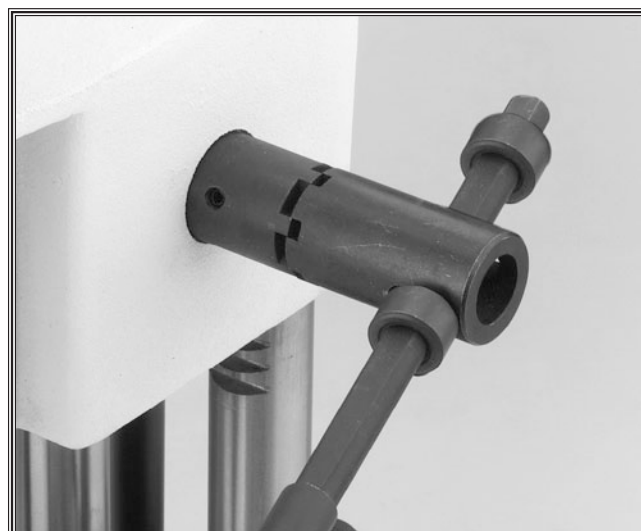
Figure 12. Indexing handle by swinging out.
