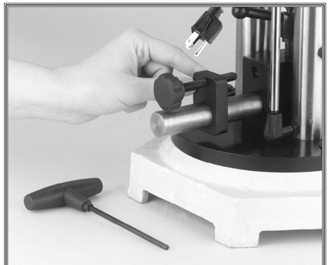
Figure 26. Setting micro-adjusting block.
