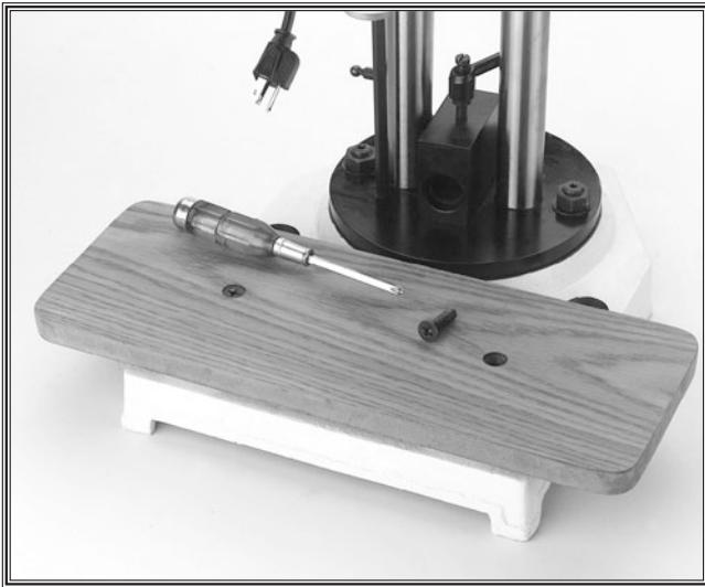
Figure 14. Work table secured with screws.
