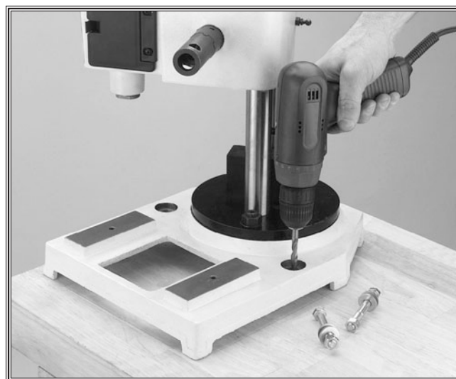
Figure 10. Using mounting holes as drill guides.
