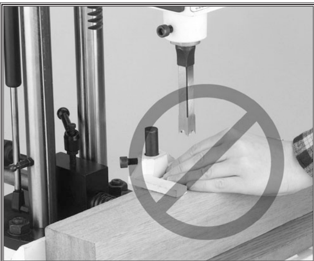
Figure 6. Never place hands under chisel.
