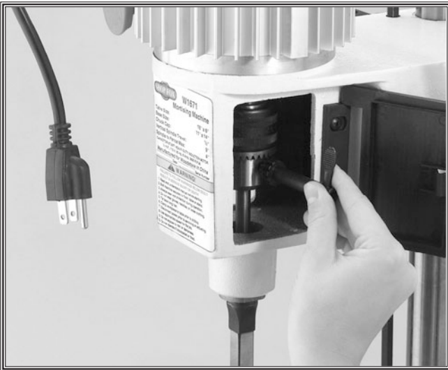
Figure 2. Unplug before changing chisels.
