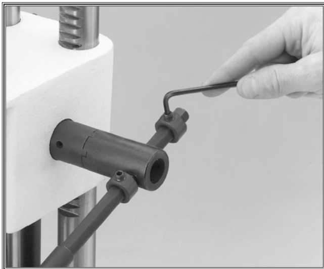
Figure 11A. Secure collar onto hand lever.
