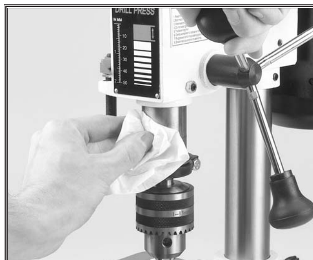
Figure 22. Clean and oil quill shaft.
