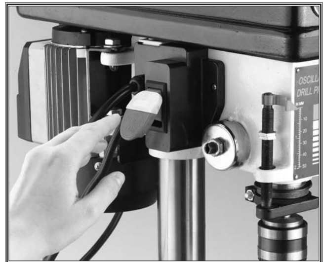
Figure 32. Hand poised over a typical stop switch.
