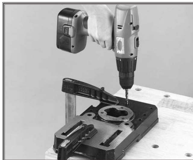
Figure 7. Using holes as a drill guide.
