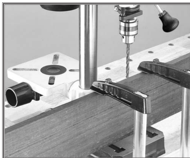
Figure 25. Table adjusted behind column.
