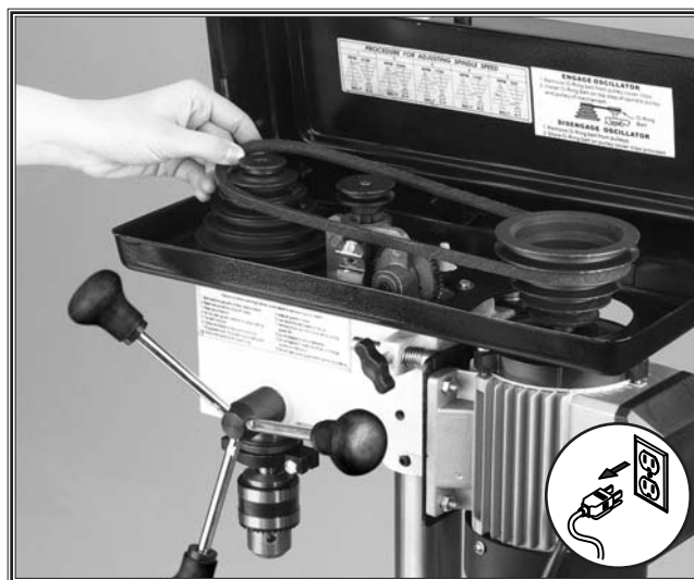
Figure 28. Adjusting belt to desired speed.
