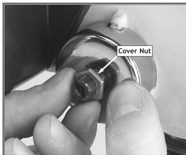
Figure 21. Hold the spring cover tightly.
