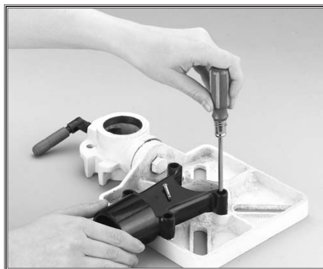
Figure 8. Installing the dust port.
