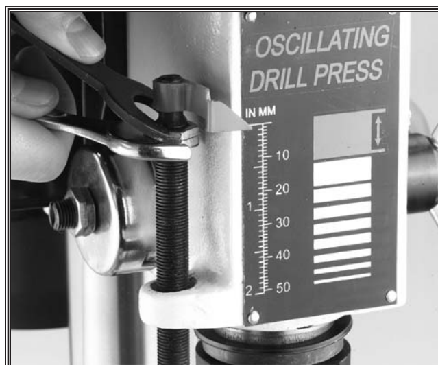
Figure 38. Back-off the depth stop nuts.
