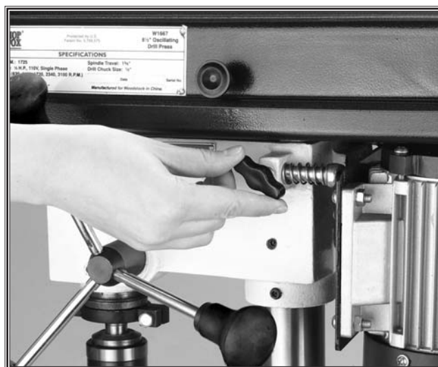
Figure 27. Loosening the lock knob.
