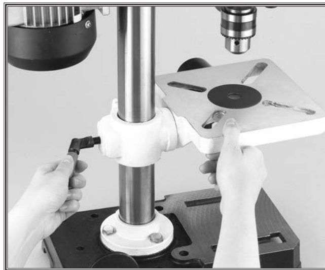
Figure 24. Support table while loosening lock.
