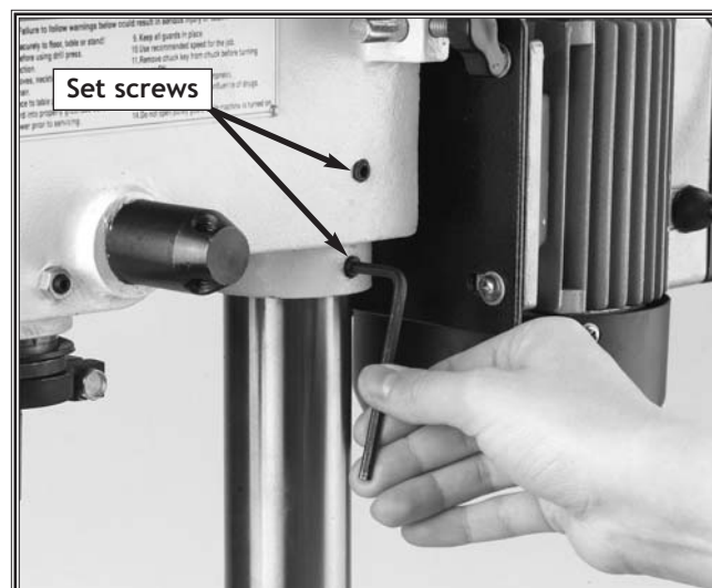
Figure 11. Securing the headstock to the column.
