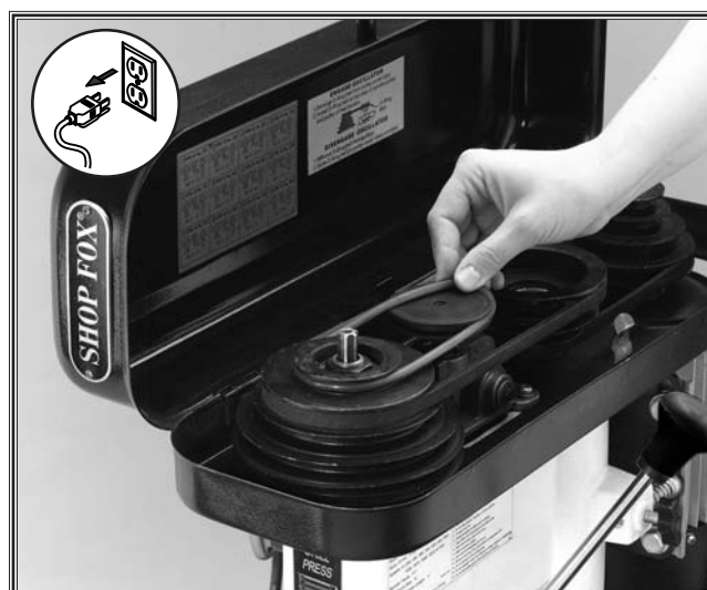
Figure 37. Stretch the belt to fit on pulleys.
