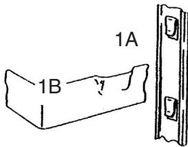
Important: The drawer must be fully closed before the lid is shut. **DO NOT** slam the drawers when the lid is shut; they will not lock and damage to lock bar tabs or lock pockets may occur. Should this happen, remove the drawer and straighten out the deformed tab with a screwdriver. For the lock pockets, a pair of pliers should be used. See (1A) lock bar tab and (1B) lock pocket.
