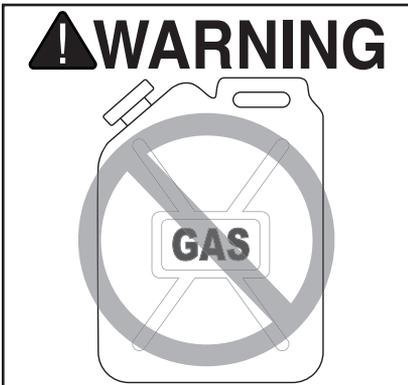
**Never use gasoline or other flammable liquids to clean this tool. Vapors in the tool may ignite, causing the tool to explode. Ignoring this warning may lead to serious personal injury or even death!**
