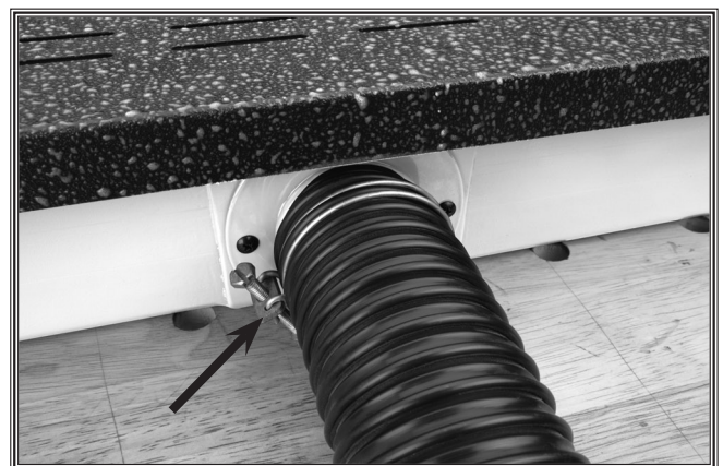
Figure 2. Dust port connected to dust collection system.
