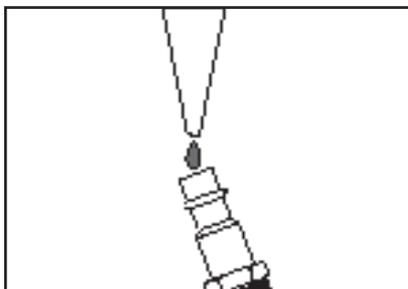
**Figure 8.** Lubricating nailer/stapler via air inlet.
