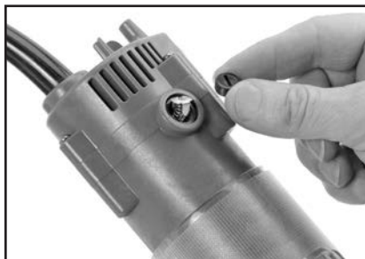
Figure 22. Replacing the motor brushes.
