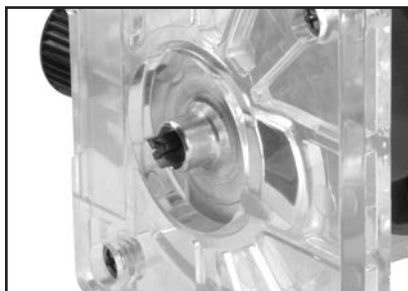
Figure 12. Router bit installed through the template guide.
